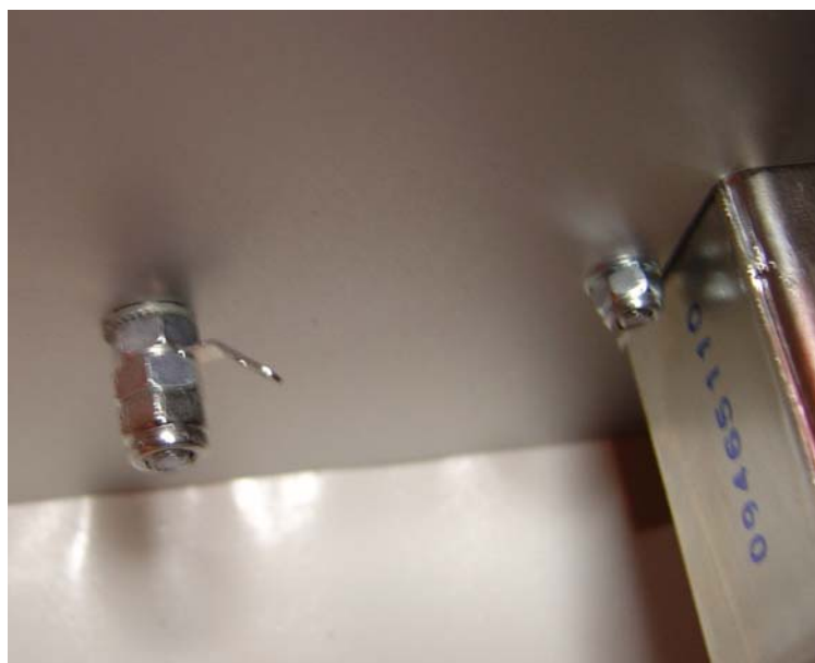
figure 11: earth connector and mains filter
