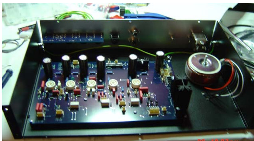
figure 14: pcb mounted to the chassis with pcb
