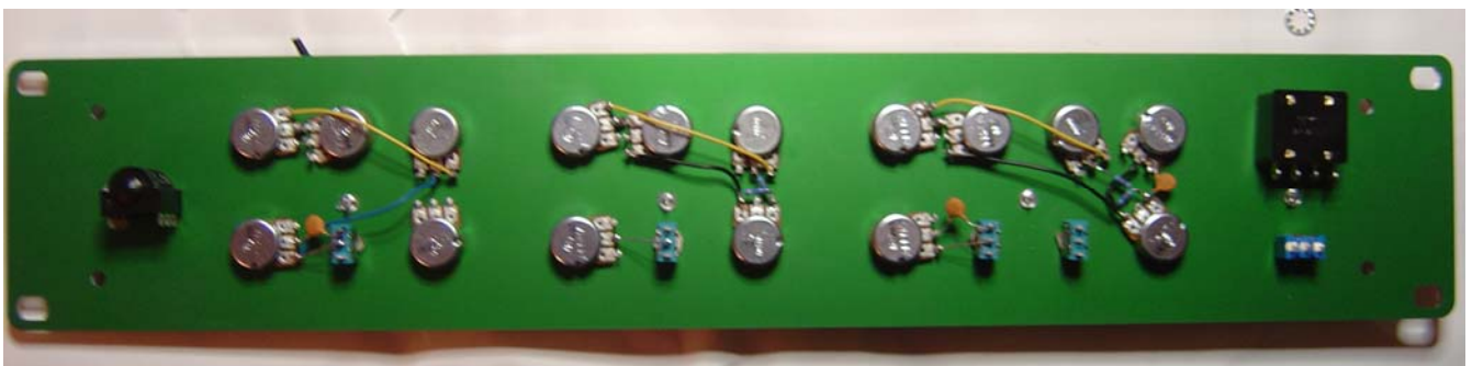
figure 19: the frontplate prewired
