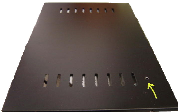
figure 4: top plate earth connector
